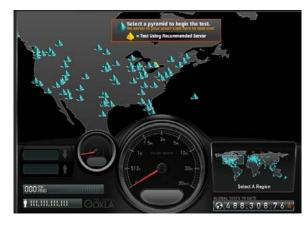
3) The speed test will give you results once it has been completed, and if your Upload speed is under 384kbps, then you will not be able to remotely access your system:
